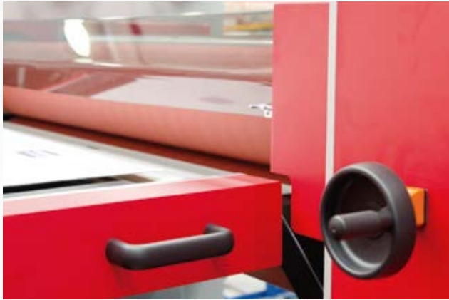
• Lamination gap adjustment.
